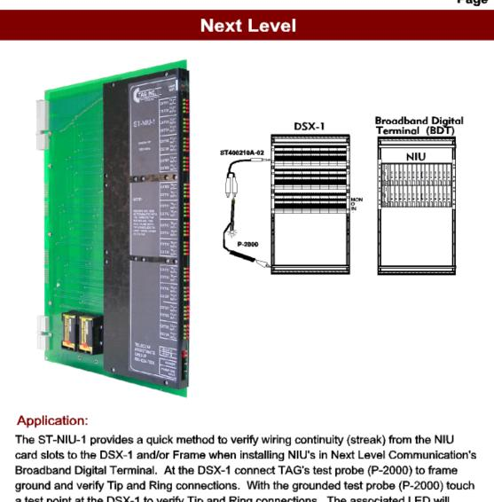
a test point at the DSX-1 to verify Tip and Ring connections. The associated LED will illuminate on the Streaker Card (ST-NIU-1). The ST-NIU-1 has 96 LED's - 48 green (tip) and 48 red (ring).
